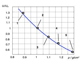
Dependence of the normalized amplitude U in the reflected signal on the density of loading liquid (1 -ethyl alcohol, 2 –distilled water, 3 -20% sugar/water, 4 -40% sugar/water, 5 -60% sugar/water)
