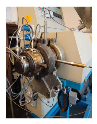
Project of ultrasonic waveguide with transducer
