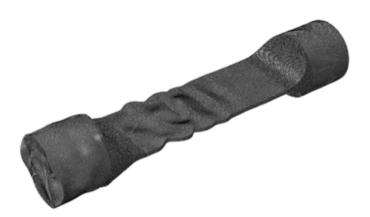
3D finite element modelling of displacement distribution in viscosity measurement waveguide
