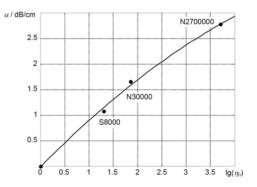
Attenuation coefficient a of the SHO wave in the aluminium wave-guide versus dynamic viscosity
