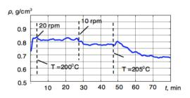
Variations of the density of the virgin PP melt for different temperatures and pressure (rpm -revolutions per minute)
