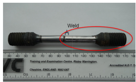
2nd reference sample after the breakage due to the development of the creep damage
