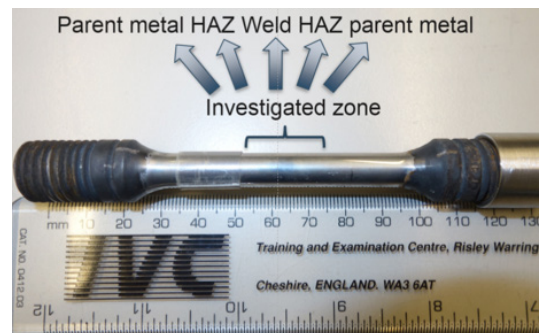
1st unbroken reference sample with the creep damage inside the weld
