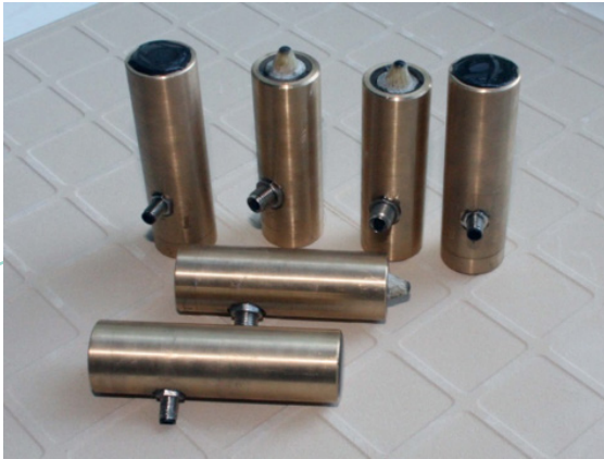
Dry contact ultrasonic transducers for testing green ceramic tiles
